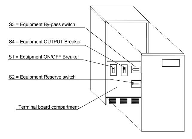
Figure 21 - 36 – 24/30/36kVA: Switches and Breakers
